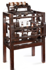
Spinning engine by Arkwright, water powered, research by Arkwright and his team of clockworkers from 1767 to 1771. Patented.
